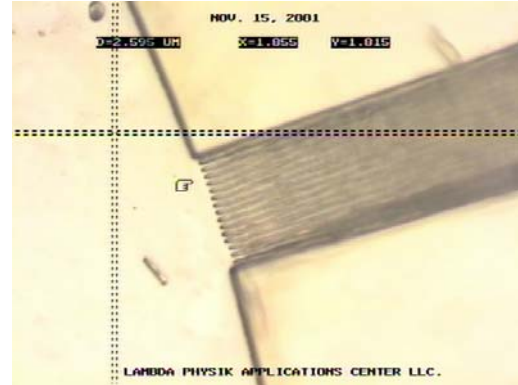
Figure 9: Polymer waveguide material etched by KrF excimer laser and Clean Lase process with \sim 290 \text{ mJ/cm}^2 . Features of less than 2 micron wide are resolved. . (Photo courtesy of Lambda Physik)
