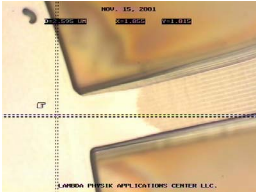
Figure 8: Polymer material etched by KrF excimer laser and Helium assist with \sim 290 \text{ mJ/cm}^2 . . (Photo courtesy of Lambda Physik)
