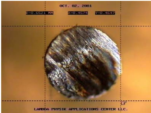
Figure 5: Beryllium/copper pin angle cut with 355 nm Nd:YAG laser. (Photo courtesy of Lambda Physik)
