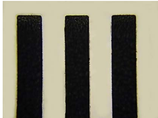
Figure 4: 200 micron slots cut into a 670 micron thick silicon with a 248 nm excimer with Clean Lase assist process. (Photo courtesy of Excitech, Inc.)
